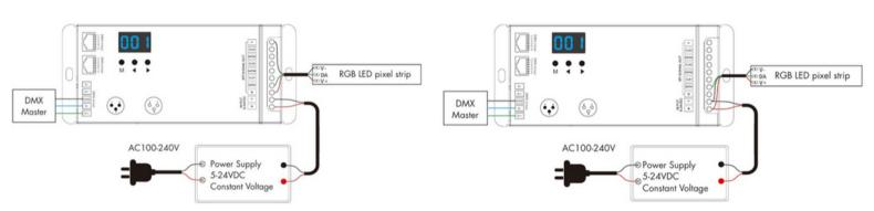
Please note that these strips are directional as indicated by the arrow on the PCB. When linking more than one strip, be sure the arrows all flow in the same way. If connecting more than 2 strips, additional power to the + and – wires will also be required every 2 additional strips. This can be delivered from the same power supply with a separate home run.
